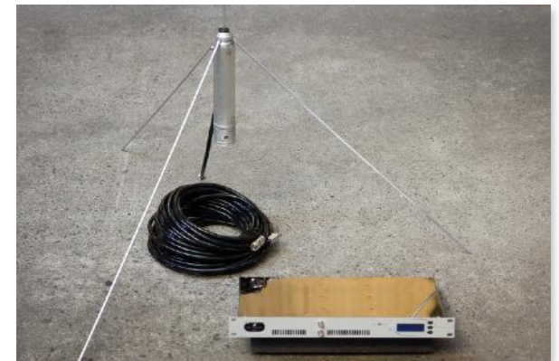
FM transmitter for the original drive-in sound
